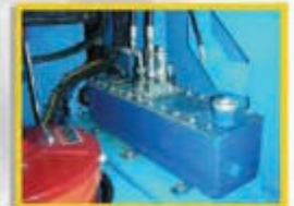
Efficient lubricator for the hammer.
